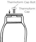
12. When the Tooling has cooled sufficiently, drill holes through the distal end of socket with a 1/4" (6 mm) drill bit, using the Thermoform Cap as a drill guide.
