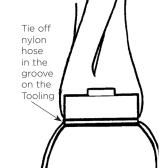
Note: Do not allow the nylon hose to extend above the tie-off groove on the Thermoform Tooling. Air leaks may occur in the finished socket if the nylon hose extends past the tie-off groove.
